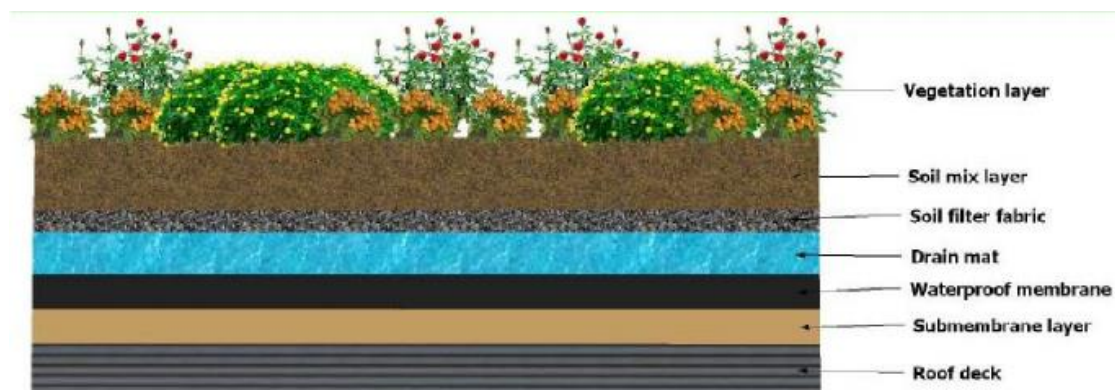
Figure 3: Typical cross section through a green roof 9
