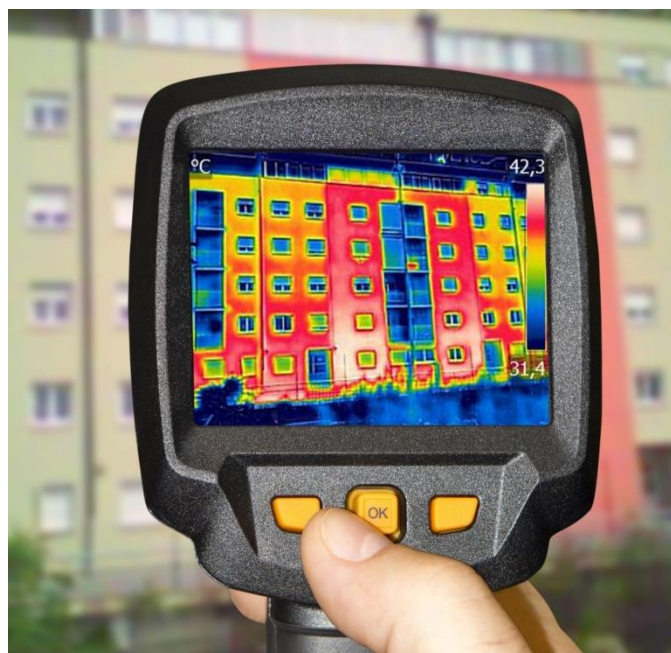
Figure 2: Thermograph picture of a building 6
